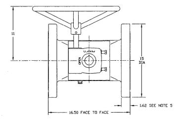
ANSI CLASS 250, CAST IRON LUBRICATED PLUG VALVE WITH GEAR AND HANDVHEEL
